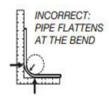
Note: RIIFO PEX-a tubing may be bent to a minimum of 8 x O.D. with approved bend support.
